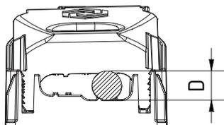
max. cable diameter D: 6.5mm
