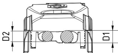
max. cable diameter D1: 6.5mm
